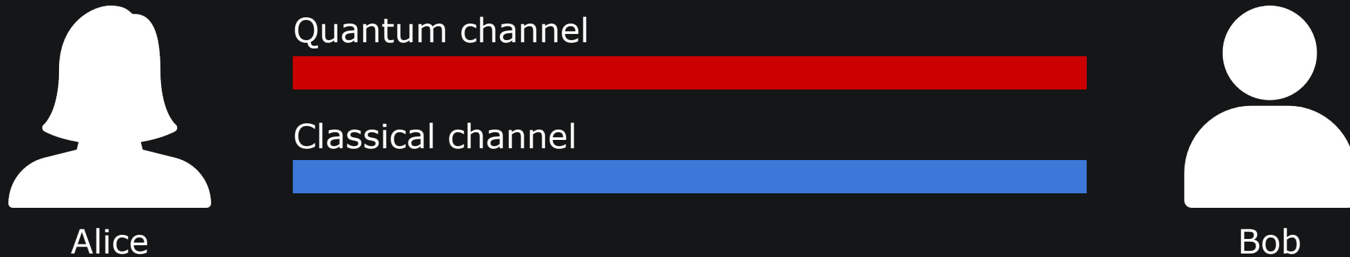
Fig 1. QKD setting. Alice and Bob are connected through a quantum channel and a classical channel [10]
